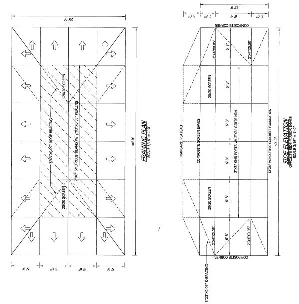
\*Contractor may change framing memeber sizes as long as new framing member meets the span requirements per attached tables.
