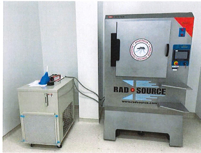
Fig. 2. Radiation machine for irradiating mosquitoes at AMCD's mass rearing facility, St. Augustine, Florida.
