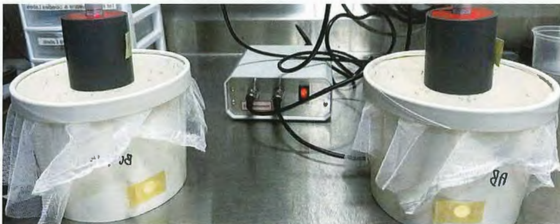
Two feeder Hemotek system with 3 mL standard reservoir, bovine (on the left), and ABM (on the right) being used to feed An. quadrimaculatus .
